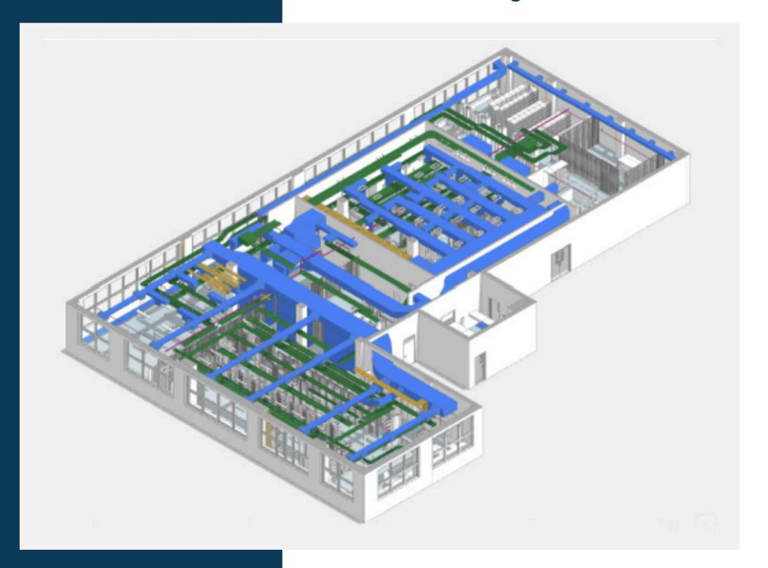
Transform your Matterport data into a LOD 200 BIM in .RVT and .DWG formats. Choose from Architecture, Interior Furniture, or MEP scopes. Specialized options apply to complex spaces like mechanical rooms or data centers.
